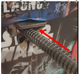
3. Now reattach the white PVC piece onto the metal bracket with the two screws. If you use a magnetic screw driver, this will be a lot easier to do as you won't drop the screws into your cabinet.
