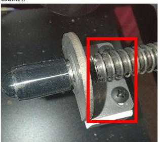
4. Now secure the plunger assembly onto the plunger using the three included machine screws. Make sure the insert the white PVC piece into the metal slider on the resister. It will pressure fit into place.
