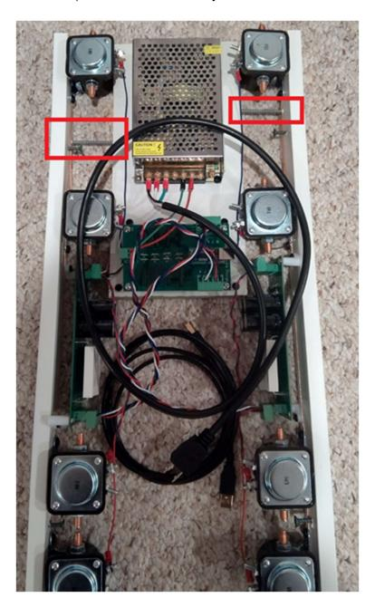
2. Unplug the wires from the main unit and install the solenoid bars into your pinball cabinet. There are four screws pre-set and ready to be used in a cabinet with ¾" walls. Be careful to check that the screws will not protrude through the sides of your cabinet before screwing them in. The orientation and positioning of the solenoid bars relative to your cabinet can be seen in the picture below:
