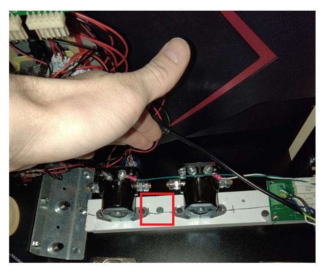
3. Plug the USB cable into your PC, the power cord into your outlet, and reconnect the main unit to the solenoid bars. Complete the software setup using the software setup instructions.
